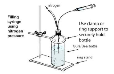
Fig. 2A Filling syringe using nitrogen pressure
