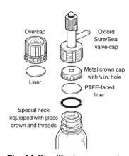
Fig. 1A Sure/Seal components
