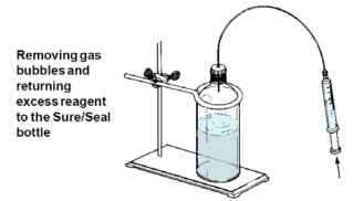
Fig. 2B Removing gas bubbles and returning excess reagent to the Sure/Seal bottle
