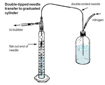
reaction apparatus. Apply nitrogen pressure as **Fig. 3B** Double-tipped needle transfer to graduated cylinder before and the measured quantity of reagent is added to the reaction flask.
