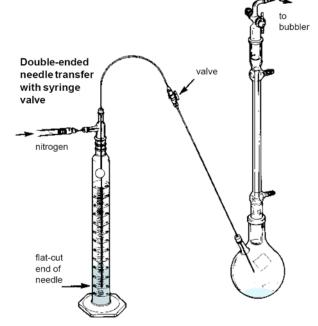
Fig. 3C Double-ended needle transfer with syringe valve
