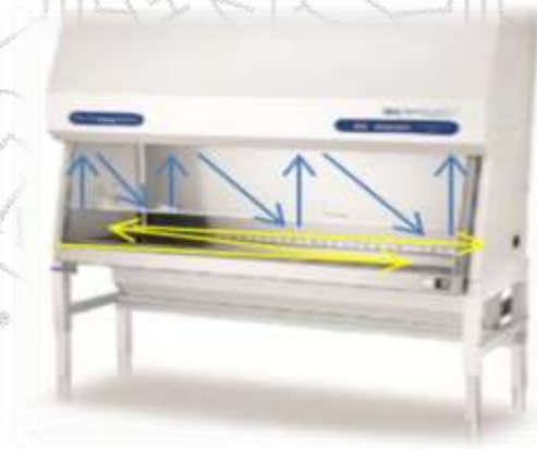
Figure 1. Cleaning work surface (yellow arrows) and sash (blue arrows)
