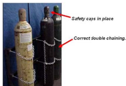
Cylinders stored and chained correctly
