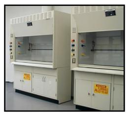
EH&S provides annual fume hood certifications for all campus fume hoods. The annual certification is a performance evaluation to ensure that the fume hood is functioning properly and protecting you from harmful materials. However, unsafe practices along with material accumulation within the hood can lead to exposure and accidents regardless if the fume hood is working properly.
