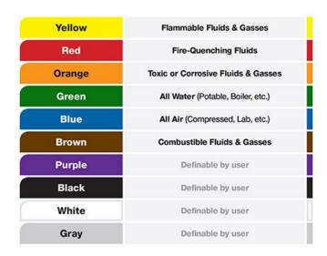
• Labels have a minimum length and letter size based upon the tubing or pipe's outer diameter and conform to the following:
