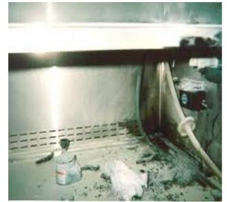
Figure 4. Fire caused by open flames in BSC
