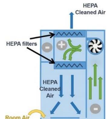
Figure 1. Side view of Class II Type A2 BSC
