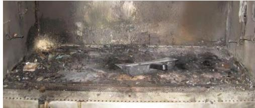
Figure 3. Fire as a result of use of open flame in a BSC
