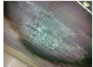
Figure 5. Damage to a HEPA filter caused by heat
