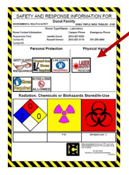
**LASER emitting equipment** are common devices used in research settings. Rooms where a LASER is located are identified in the "**physical hazards**" section of the room posting.
