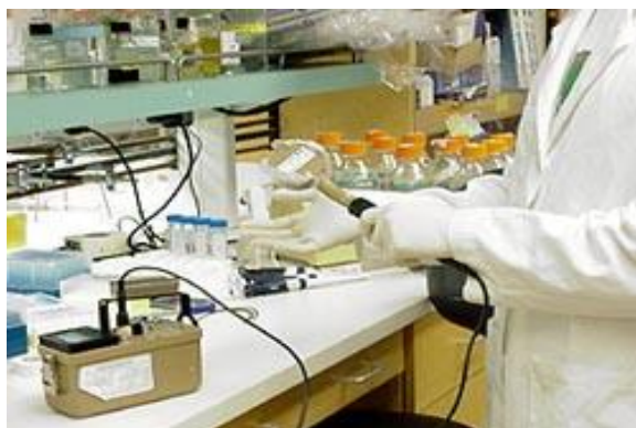
Performing a survey with a GM Survey Instrument
